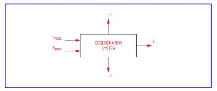
Figure 2.1.1 Cogeneration System Inputs and Outputs
