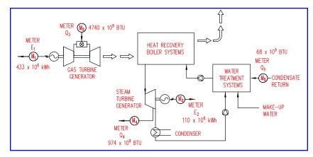
Figure 2.1.2 Natural Gas-Fired Combined Cycle in Cogeneration Mode
