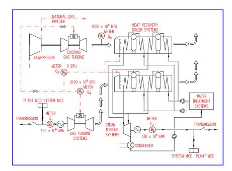
Figure 2.1.4 Enhanced Combined Cycle System at a Natural Gas
